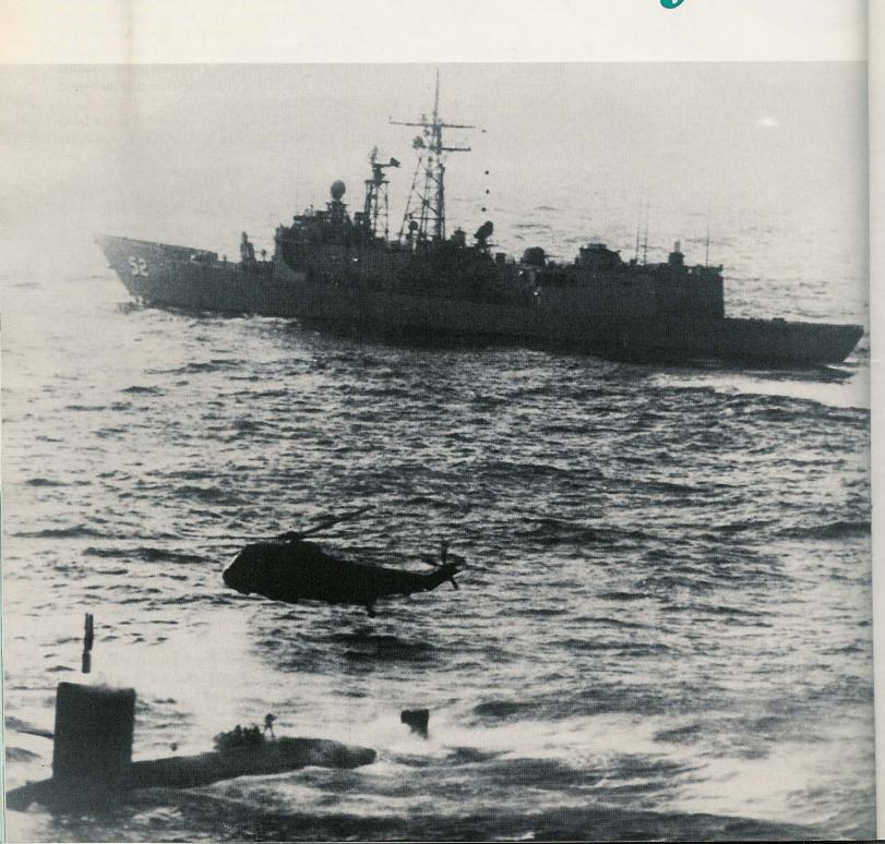
ON April 24, 1988, USS *Bonefish* (SS-582) experienced a serious fire that began in high-voltage DC cable in a midship compartment. The fire rapidly spread upward, producing fumes and dense smoke. Many of the 92 crewmen aboard were affected and barely managed to escape to the stricken sub's deck and sail to await rescue by nearby ships and helicopters.
