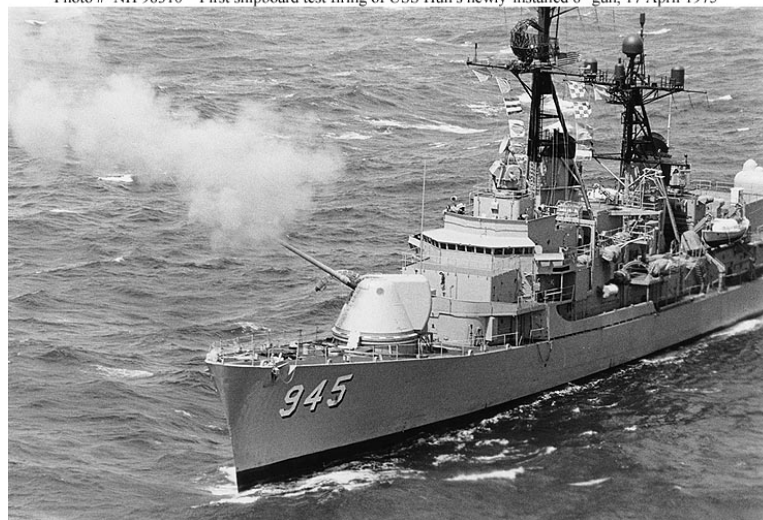
Photo # NH 98310 First shipboard test firing of USS Hull's newly-installed 8" gun, 17 April 1975
